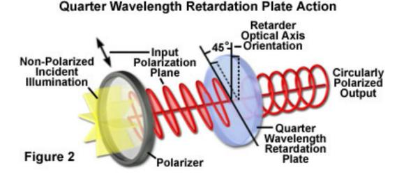
Modifying wave polarization in a quarter wave plate (1)
