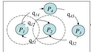
$$\mathbf{Q} = \begin{bmatrix} -(q_{12} + q_{14}) & q_{12} & 0 & q_{14} \\ q_{21} & -q_{21} & 0 & 0 \\ 0 & q_{32} & -q_{32} & 0 \\ 0 & 0 & q_{43} & -q_{43} \end{bmatrix}$$
