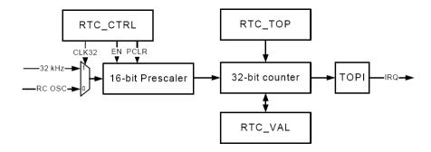
The prescaler can be used to set the base frequency for the RTC. The base frequency is given by the following formula:  $f_{RTC} = 2^{-(PSEL+1)} \cdot (f_{RC} \text{ or } 32 \text{ KHz})$
