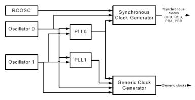
The CPU and the different buses on the chip may run at different clock speeds. By default, the CPU runs off the RC oscillator (~115kHz) and hence is quite slow. By
