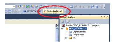
Click on this *No tool selected* button to open the project properties window. Select the JTAGICE mkll as debugger/programmer. Close project properties.
