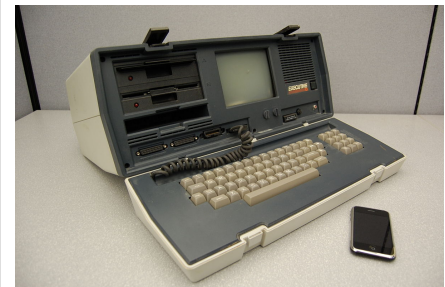
An Osborne Executive portable computer, from 1982 with a Zilog Z80 4MHz CPU, and a 2007 Apple iPhone with a 412MHz ARM11 CPU. The Executive weighs 100 times as much, is nearly 500 times as large by volume, costs approximately 10 times as much (inflation adjusted), and has 1/100th the clock frequency of the smartphone.
