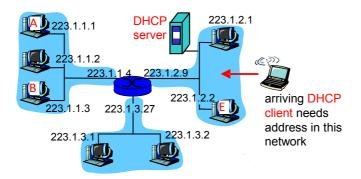
In the simplest case, four DHCP messages will be exchanged according to the figure below. Name these four DHCP messages (message type) and fill in the missing fields in each message. You can assume that the subnet to which the DHCP client arrives is a /24 network and that all addresses below 223.1.2.10 are occupied. Based on that, you can let the DHCP server hand out a suitable IP address. You also have to select reasonable transaction IDs.
