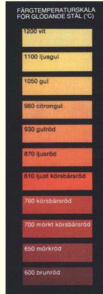
Chart to estimate steel temperature in steelworks.
