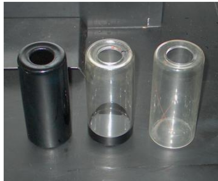
Figure : RTFO Samples (left - after aging in the RTFO, center - before aging in the RTFO, right - empty sample jar)
