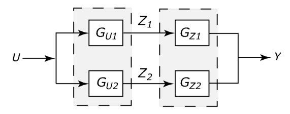
$$\begin{pmatrix} Z_1(s) \\ Z_2(s) \end{pmatrix} = \begin{pmatrix} G_{U1}(s) \\ G_{U2}(s) \end{pmatrix} U(s), \qquad Y(s) = \begin{pmatrix} G_{Z1}(s) & G_{Z2}(s) \end{pmatrix}$$
