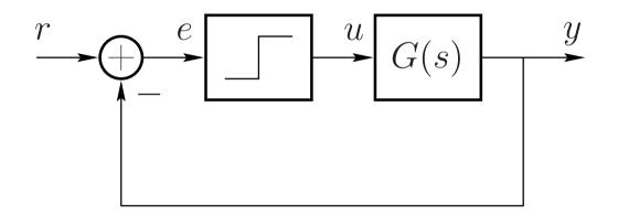
The relay corresponds to infinite high gain at the switching point
