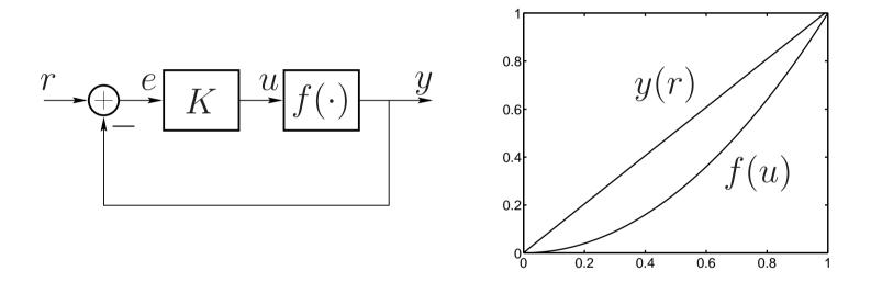
Linearization of  $f(u) = u^2$  through feedback. The case K = 100 is shown in the plot:  $y(r) \approx r$ . The Sensitivity Function  $S = (1 + GF)^{-1}$
