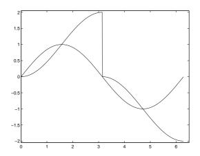
(b) The output of an integrator with sinusoidal input is
