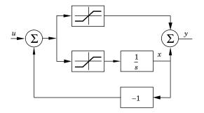
The system is a jump and rate limiter: y is equal to u if u changes slowly. If u makes an abrupt change, then y converges to u after a while. Conclude this by simply deriving the equations for the system for  $|u-x| \leq 1$  and for  $|u-x| \geq 1$ , when u makes a step change.
