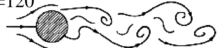
Oscillating Karman vortex street wake (C)
