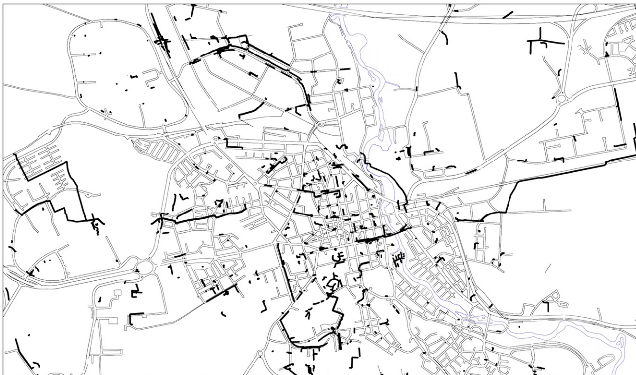
Fig. 1. Map of disconnected low- and medium-voltage power cables (bold black lines) in the city centre of Linköping retrieved from the power grid manager's GIS data. The scale of the map is 1:20000.
