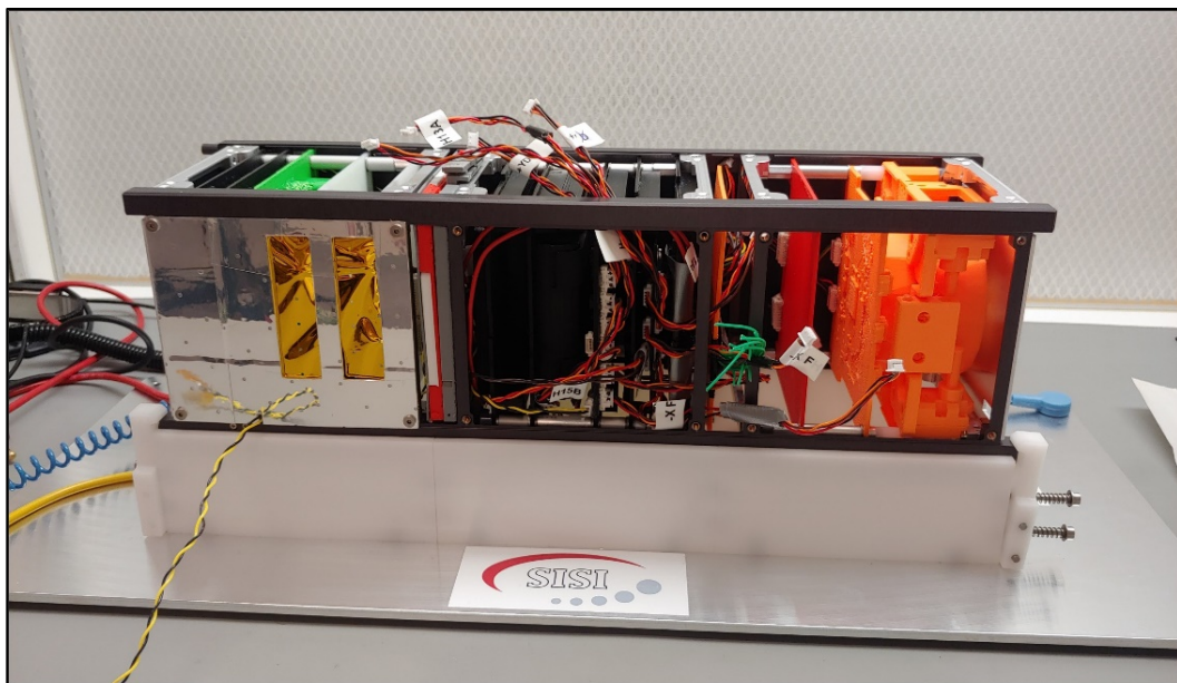
Figure 3 The MIST flight structure with simulated subsystems.
