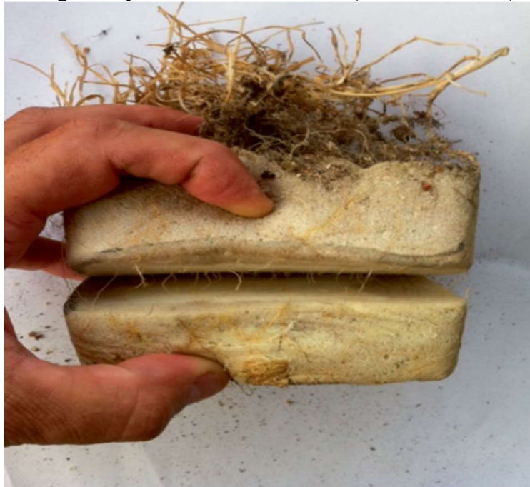
Figure. 4: Experimental hydroponic foam layer beneath the growing greenery, providing plant-available water while retaining stormwater (Sutton, R. K. (Ed.). 2015).
