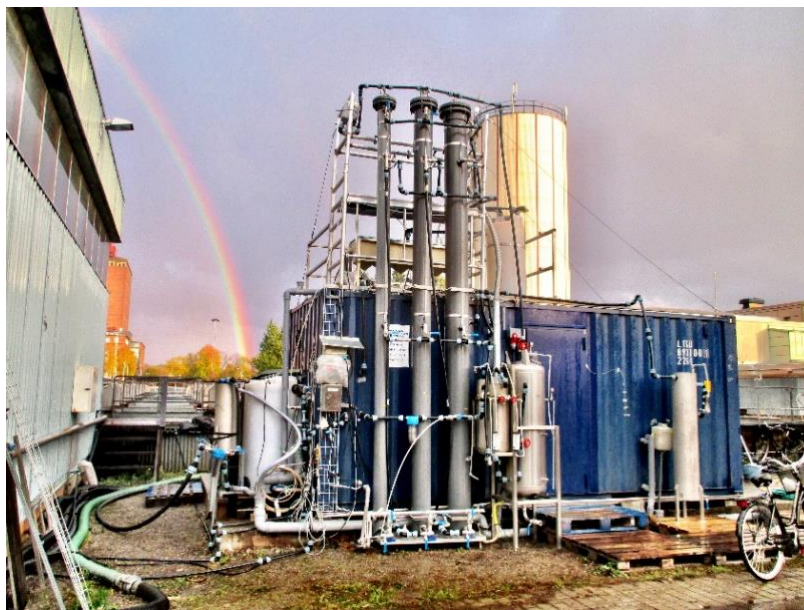
Figure 4. Mobile pilot plant for removal of pharmaceutical residues from effluent of waste-water treatment facilities.
