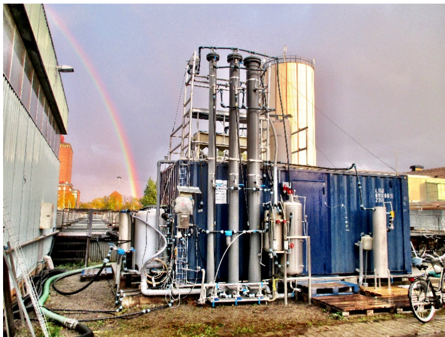
Figure 2. Mobile pilot plant for removal of pharmaceutical residues from effluent of waste-water treatment facilities.
