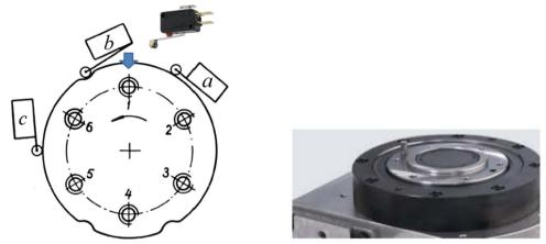
One wants to indicate the table position with a numeric display that has inputs for binary code  $y_2y_1y_0$ . The display also has an enable input *EN*. To show the numbers it is required that EN = '1', the display is off when EN = '0'.
