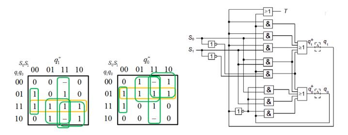
All state transitions have Haming distance 1 if Gray code is used. Hazard cover in yellow is needed.  $q_0^+ = S_0 S_1 + q_0 \overline{S}_0 \overline{S}_1 + \overline{q}_1 S_0 + \overline{q}_1 S_1 + \overline{q}_1 q_0$   $q_1^+ = S_0 S_1 + q_0 \overline{S}_0 \overline{S}_1 + q_1 S_0 + q_1 S_1 + q_1 q_0$   $T = q_0 + q_1$
