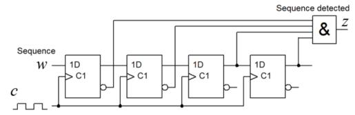
**a**) (1p) Which bit sequence is detected?
