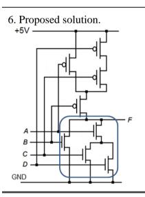
Pulldown net  $\overline{F} = B + A \cdot (C + D)$   $\Rightarrow F = \overline{B + A \cdot (C + D)} = \overline{B} \cdot \overline{A \cdot (C + D)} =$   $= \overline{B} \cdot (\overline{A} + (\overline{C + D})) = \overline{B} \cdot (\overline{A} + \overline{C} \cdot \overline{D}) = \overline{B} \cdot \overline{A} + \overline{B} \cdot \overline{C} \cdot \overline{D}$
