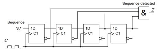
**a**) (1p) Which bit sequence is detected?
