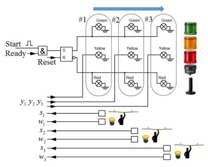
**a**) (a+b=1p) (**Green**) A short pulse Start = 1 can start the assembly line *if* Ready = 1. Design a circuit that provides signal Ready = 1 if *none* of the stop signals  $s_1 s_2 s_3$  are 1.
