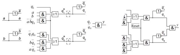
d) An active low Reset could be inserted with two and-gates as the initial state A has the code 00.
