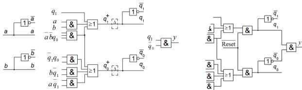
d) An active low Reset could be inserted with two and-gates as the initial state A has the code 00.
