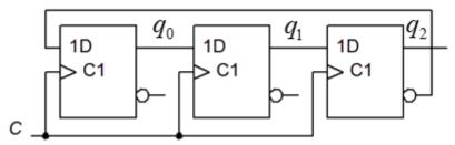
A synchronous counter starts in the state  $q_2q_1q_0 = 000$ . What will the state be after **four** clock pulses?  $q_2q_1q_0 = ?$
