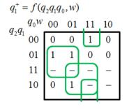
$$\begin{aligned} q_2^+ &= q_1 q_0 w \\ q_1^+ &= q_1 q_0 + q_2 w + q_1 q_0 w \\ q_0^+ &= q_1 q_0 w + q_2 q_1 q_0 w \end{aligned}$$
