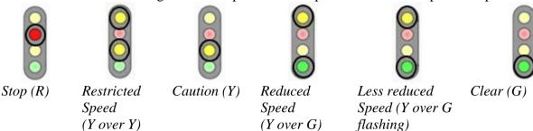
Design a *signal decoder*, a combinatorial logic network, which uses a three-bit mode signal M ( $m_2$   $m_1$   $m_0$ ) to generate output signals controlling four colored lights ( $y_1$  r  $y_0$  g).
