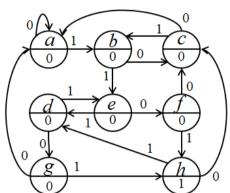
**b**) (4p) A sequence detector is expected to detect each occurrence of a sub-sequence ... 1101 ... within a sequence of bits received by the input *w*.
