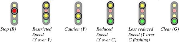
Design a *signal decoder*, a combinatorial logic network, which uses a three-bit mode signal M ( $m_2$   $m_1$   $m_0$ ) to generate output signals controlling four colored lights ( $y_1$  r  $y_0$  g).
