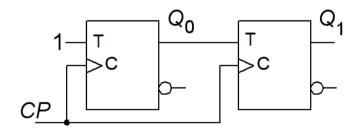
A synchronous counter with **T** flip-flops in the figure starts in the state  $Q_1Q_0 = 00$ . Give its sequence of states for the following four clock pulses.
