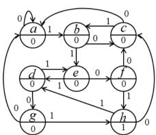
**b**) (4p) A sequence detector is expected to detect each occurrence of a sub-sequence ... 1101 ... within a sequence of bits received by the input *w*.
