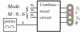
Mode 1...6,  $m_2 m_1 m_0 001 ... 110$  (in binary), select signals for incrementally increasing allowable speed according to the standard shown in the figure above.
