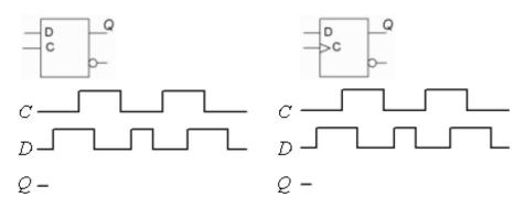
Complete the timing diagram for the D-latch and D-flipflop by drawing signal Q for booth cases. Draw the figure so that it is clear **what** is causing the changes in the Q!
