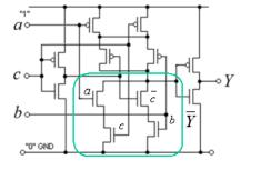
$PDN: \quad \overline{Y} = ac + b\overline{c}$  $\Rightarrow \overline{\overline{Y}} = Y = ac + b\overline{c}$
