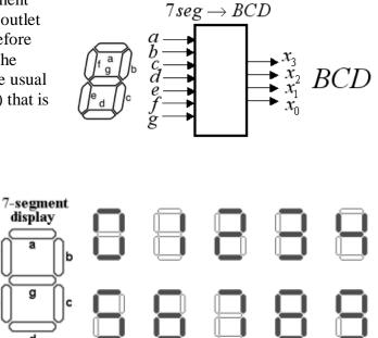
**a)** (1p) Set up the **truth table** for the ten BCD numbers. Black segment is "1" in figure.  $(x_3x_2x_1x_0)_{BCD} = f(abcdefg)$
