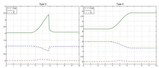
Note the small entropy-violating "shocklet" in type 3... the entropy fix should be strengthened
