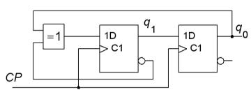
A synchronous counter as shown above starts with the state  $q_1q_0 = 00$ . Specify the **count sequence** for the next four clock pulses.
