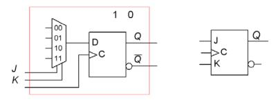
Show (draw) how to make a JK flip-flop of the D flip-flop and a 4: 1 multiplexer. In addition to Q and its inverse, there are constants 1 and 0 available. A copy of the figure is also on the submission sheet.
