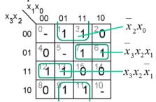
$$Y_{\min} = \overline{x}_2 x_0 + \overline{x}_3 x_2 x_1 + x_3 x_2 \overline{x}_1$$
