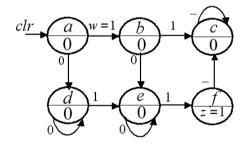
$$clr \rightarrow a \quad \begin{array}{c|ccc} 0 & w_1 & z \\ \hline d & b & 0 \\ b & e & c & 0 \\ c & c & c & 0 \\ d & d & e & 0 \\ e & e & f & 0 \\ f & c & c & 1 \end{array}$$
