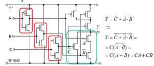
The circuit has three inverters that first inverts the signals AB and C to  $\overline{ABC}$  before they proceed.
