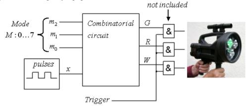
You shall construct a combinatorial circuit for a signal lamp for traffic control tower (emergency). With an 8-position binary coded switch
