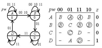
The states can be coded with the gray code. Two of the don't care entries occur because the signal w is slow and then always will be w = 1 during the pulses from p. The other two don't care entries occur because input signala can have no double changes.
