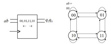
a) (1p) Finish the initiated state diagram. Map the condition for all state transitions. b) (2p) Write state table based on the state diagram.  $q_1^+q_0^+ = f(q_1q_0, ab)$ Derive minimized expressions for the next state.  $q_1^+ = f(q_1q_0, ab)$   $q_0^+ = f(q_1q_0, ab)$
