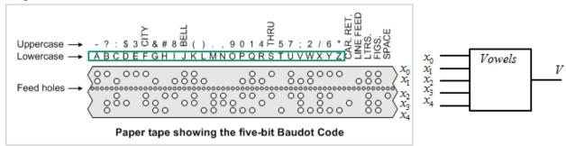
The figure shows an punched tape with the Baudot code. Your task is to make a decoder for vowels (our Swedish vowels Å Ä Ö are *not* included) that provides the output V=1 only when the code is corresponding to a vowel. Assume that the paper tape to read is edited so that only the English alphabet letters **A** ... **Z** are appearing (letters from the line "Lowercase"). No special characters (Car. Return, Line Feed, Ltrs ...) can occur. Consider Y as a vowel. Hole = 1, no hole = 0.
