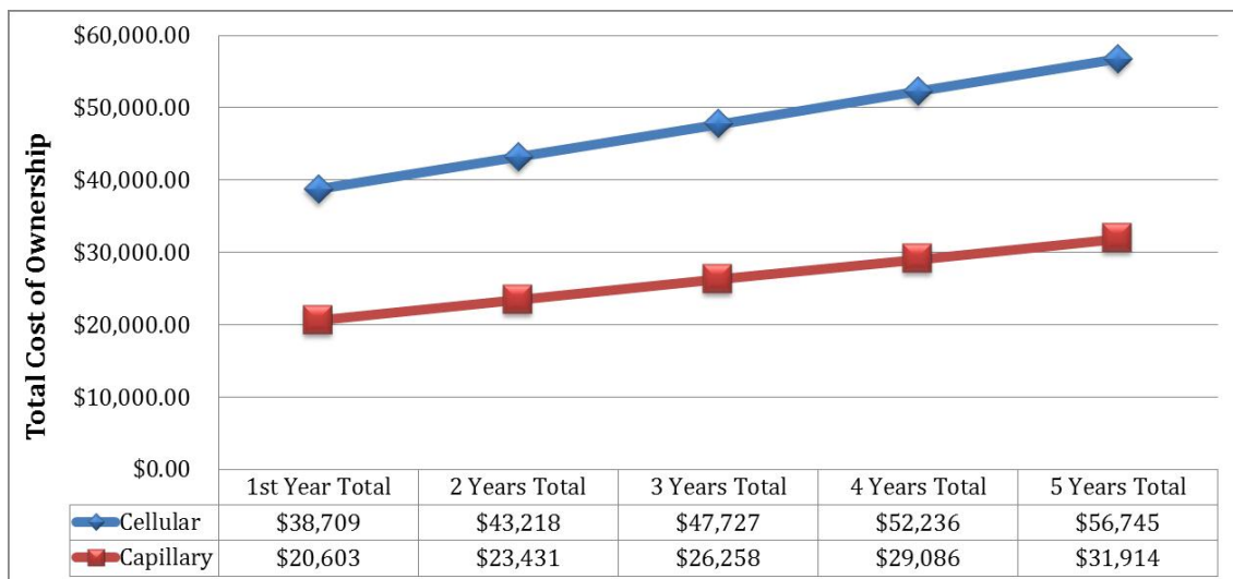
Figure 4.7 Cost comparisons of cellular and capillary solutions in a 5-year period for Scenario B
