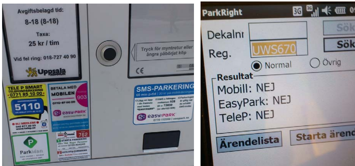
Figure 6. Ticket machine illustrating multiple payment solutions for parking (left) and a snap shot showing the user interface of the handheld device for the ticket control staff (right).
