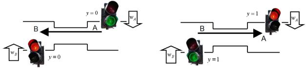
At roadworks when forced to make a path so narrow that only cars in one direction at a time can pass, usually putting up traffic signals. You will design a synchronous sequential circuit, in the form of a positive edge-triggered Moore machine with D flip-flops for controlling such a traffic signal.
