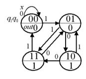
c) Multiplexers are using the select variables x and  $q_0$  so therefore we change the variable order of the encoded state table.
