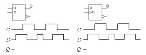
Complete the timing diagrams for the D-latch and D-flipflop by drawing signal Q for booth cases. Draw the figure so that it is clear **what** is causing the changes in the Q! 9. 1p/0p
