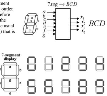
c) (2p) Draw the karnaugh maps for the four BCD-code bits and derive the **minimized expressions** for  $x_3 x_2 x_1 x_0$  in SoP-form. Segment combinations that never occurs should be exploited as don't care. (With the excluded segments in the truth table, the number of variables will be manageable).
