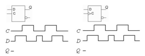
Complete the timing diagram for the D-latch and D-flipflop by drawing signal Q for booth cases. Draw the figure so that it is clear **what** is causing the changes in the Q!
