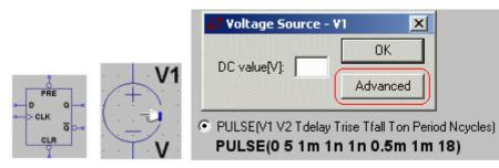
Component. 74HCT74. Component. voltage. Then Change the voltage source with Advanced and PULSE to get a number of clock pulses.
