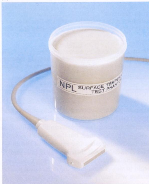
Fig. 12.3 (a) Diagram of a thermal test object. The temperature rise in the middle of the tissue-mimicking material (TMM) is measured with a small thermocouple of less than 0.5 mm in diameter. (b) Photograph of a commercial thermal test object for testing surface temperature rise against the limits specified by the IEC.
