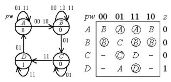
The states can be coded with the gray code. Two of the don't care entries occur because the signal w is slow and then always will be w = 1 during the pulses from p.
