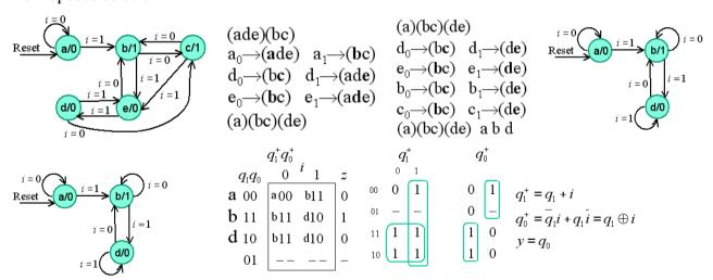
State encoding is free, except that a must have the code 00 as we use asynchronous reset.
