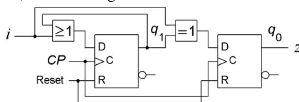
12. (5p) Asynchronous edge triggered pulse gate
