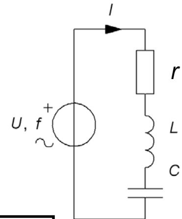
$$\text{Im}[\underline{Z}] = \omega L - \frac{1}{\omega C} = 0 \quad \Rightarrow \quad \omega_0 = \frac{1}{\sqrt{LC}} \quad f_0 = \frac{1}{2\pi\sqrt{LC}}$$
