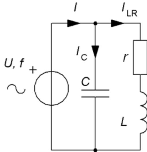
$$\omega_0 C = \frac{\omega_0 L}{r^2 + (\omega_0 L)^2} \Rightarrow \omega_0^2 = \frac{1}{LC} - \frac{r^2}{L^2} \quad \omega_0 = 2\pi f \Rightarrow f_0 = \frac{1}{2\pi} \sqrt{\left( \frac{1}{LC} - \frac{r^2}{L^2} \right)}$$
