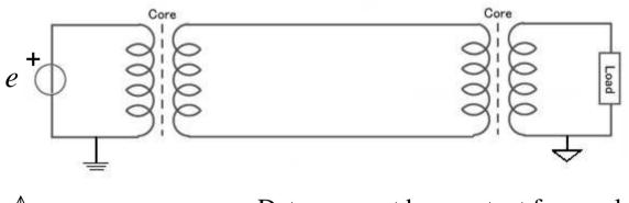
Data may not be constant for any length of time because "direct voltages" can not pass through transformers!
