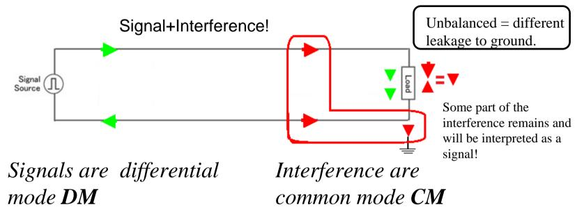
An unbalanced equipment has "closer" to the ground for one conductor, a part of the interference then takes that way – the remaining rest of the interference is perceived as if it were the signal.
