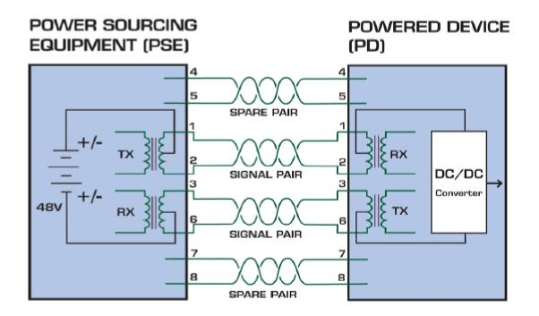
• The "smart" way that *does'nt* use the "spare pairs" ...
