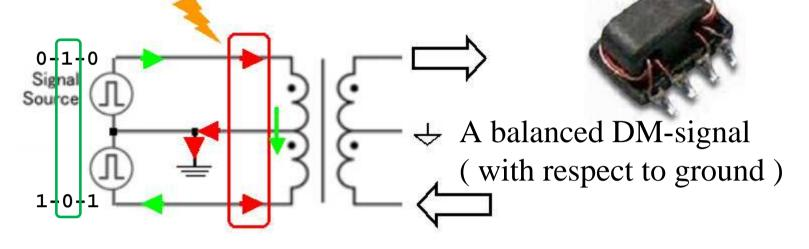
The transmitted data signal consists of two "opposing" pulses which together run a current through both winding halves. Local interference occurs common mode and will instead be led to ground, and never reach the transformer's secondary side.
