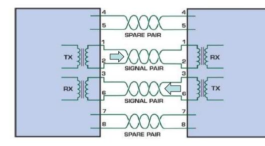
4 signal pairs, two spare wires. What can you use the spare wires to?
