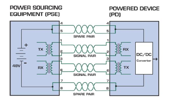
**Spare wires?** • power over ethernet
