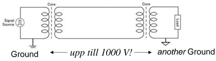
The transformers isolate different devices from each other even if the ground potentials should happen to differ by up to 1000 V!
