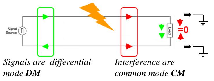
• Signals are **differential mode**, they have different current direction in the they have different current direction in wire and return wire.
