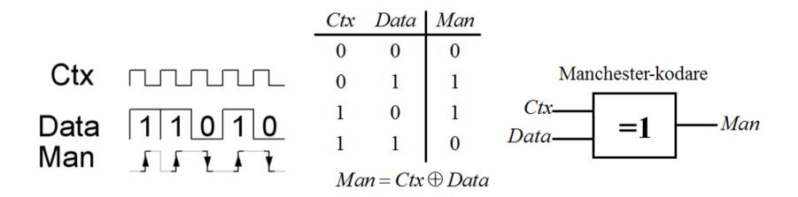
It is sufficient with a single exclusive OR gate for producing a Manchester signal from the data and clock pulses!
