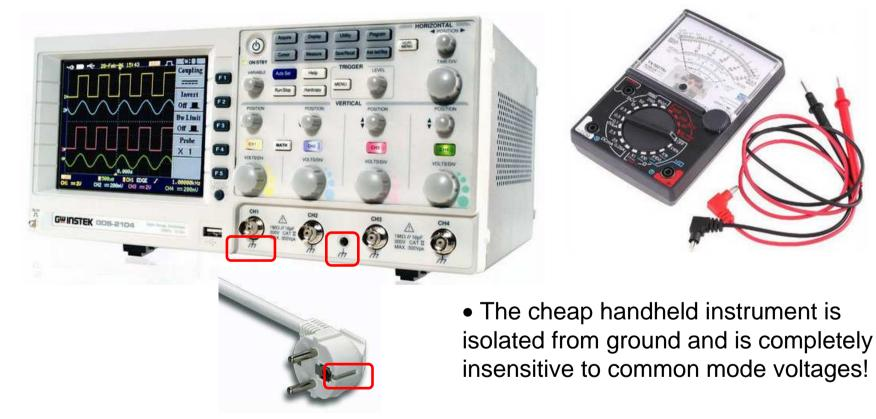
• The expensive oscilloscope has grounded inputs, thus becoming sensitive to common mode interference!
