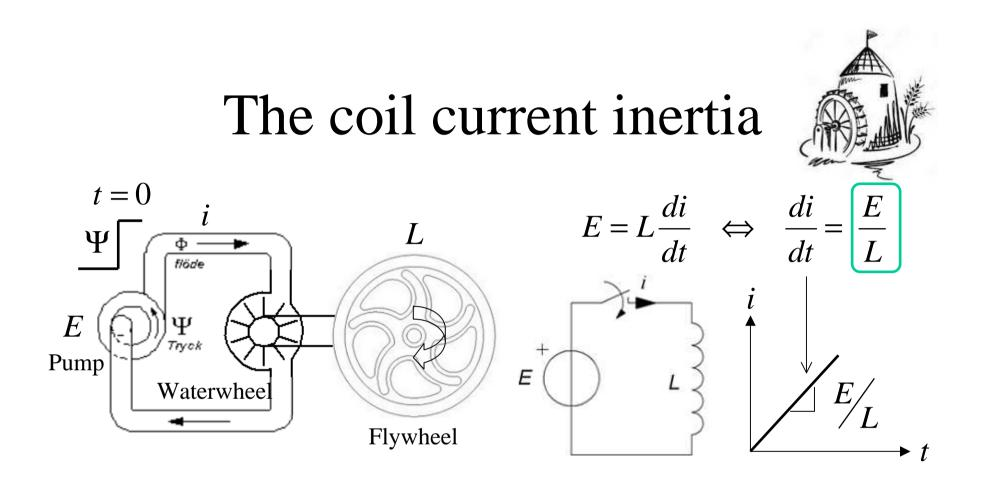
The inductor has **current-inertia**. The current can not change immediately. A fluid analogy: The inductor is a water mill with a flywheel.
