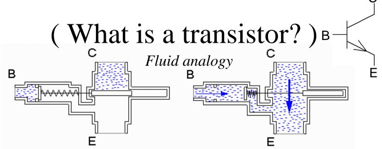
The classic bipolar transistor, is earlier development than the MOS transistor. A small "base current"  $I_{\rm B}$  can control up to 100 times ( $h_{\rm FE}$ ) bigger "collector current"  $I_{\rm C}$ .
