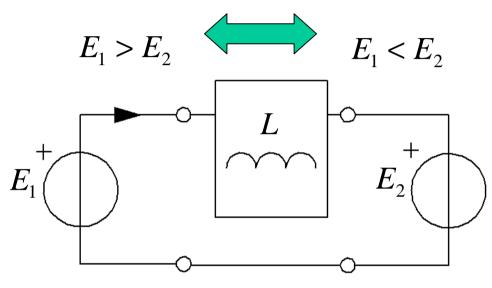
With an inductor one can transfer energy from a larger emf to a smaller,  $E_1 > E_2$ , **Step Down**, but also from a smaller emf to a larger,  $E_1 < E_2$ , **Step Up**. This in theory is completely without losses.
