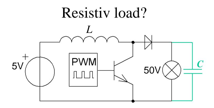
The current to the load will flow intermittently only during  $t_{off}$ , so the voltage needs to be smoothed with a capacitor *C*.
