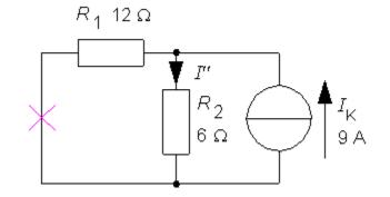
$$I'' = I_{K} \cdot \frac{R_{1}}{R_{1} + R_{2}} = 9 \cdot \frac{12}{12 + 6} = 6$$
