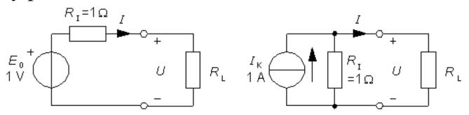
We compare the two models with external resistor  $R_L = 1 \Omega$
