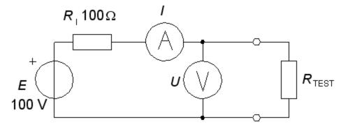
$$R_{\text{TEST}} = 10 \text{ k}\Omega \ I \approx 10 \text{ mA} \ U \approx 100 \text{ V} \ (=99,0099 \text{ V})$$
