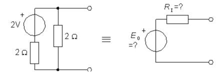
$E_0$  becomes the same as the given two-terminal open circuit voltage.
