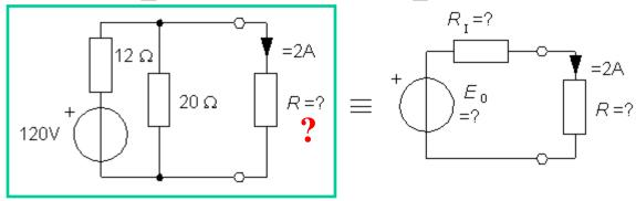
What value should *R* have for the current through the resistor will be 2A? If *R* was connected to a two-terminal equivalent the problem would be elemental.
