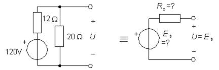
If you do not turn down the voltage sources we see that  $E_0 = U$  = open circuit voltage:
