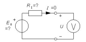
$R_{\rm I}$  is then determined by loading the circuit with an adjustable resistor so that U drops to  $E_0/2$ . Then the adjustable resistance has the same value as the internal resistance.  $R = R_{\rm I}$ .
