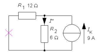
$$I'' = I_{K} \cdot \frac{R_{1}}{R_{1} + R_{2}} = 9 \cdot \frac{12}{12 + 6} = 6$$
