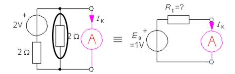
After an imagined short circuit, the internal resistance  $R_{\rm I}$  can be calculated with help of the imagined short circuit current  $I_{\rm K}$ .
