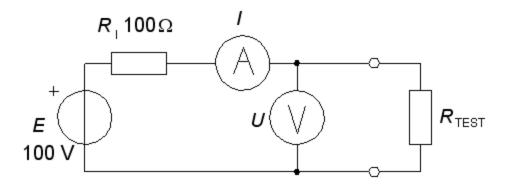
$$R_{\text{TEST}} = 1\Omega \ I \approx 1 \text{A} \ U \approx 1 \text{ V} \quad (=0.9901 \text{ A})$$
