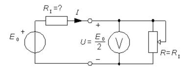
• The adjustable resistance can then be measured with a  $\Omega$ -meter (=  $R_{\rm I}$ ).
