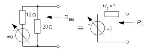
If all voltage sources would be halved in the original circuit then of course  $E_0$  in the two-terminal equivalent is also halved. Therefore, if one "turn down" all voltage sources all the way to (almost) "0" in both circuits, there will only be resistors left, then one can see that  $R_{\rm I}$  is equal to the replacement resistance in the original circuit  $R_{\rm ERS}$ :
