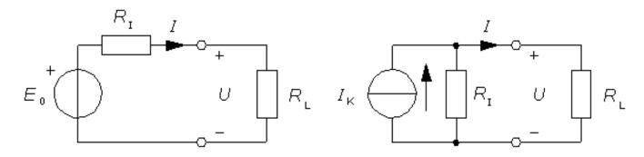
**Thévenin** voltage source model, and **Norton** current source-model for two-terminal circuits.
