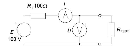
An unknown voltage source is to be tested with some test resistors.
