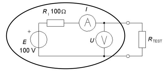
An unknown voltage source is to be tested with some test resistors.
