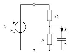
$$\frac{\underline{I}_{C}}{\underline{U}} = \frac{j\omega C}{2 + j\omega RC} \quad \frac{I_{C}}{U} = \frac{\omega C}{\sqrt{4 + (\omega RC)^{2}}} \quad \arg\left(\frac{\underline{I}_{C}}{\underline{U}}\right) = 90^{\circ} - \arctan\left(\frac{\omega RC}{2}\right)$$
