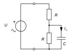
$$\frac{\underline{I}_{C}}{\underline{U}}\left\{\omega=0\right\} = \frac{0 \cdot j}{2+0 \cdot j} = 0 \quad \frac{\underline{I}_{C}}{\underline{U}}\left\{\omega=\infty\right\} = \frac{1}{R}$$
