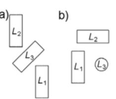
In the figure to the right b) the inductors are mounted three dimensional so that there are no shared power magnetic lines.
