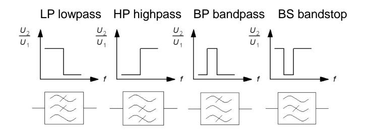
BP and BS filters can be seen as different combination of LP and HP filters.
