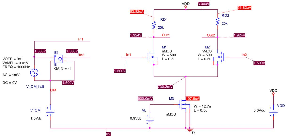
With this arrangement of input voltage source we can change common mode and differential mode input voltages independently of each other.
