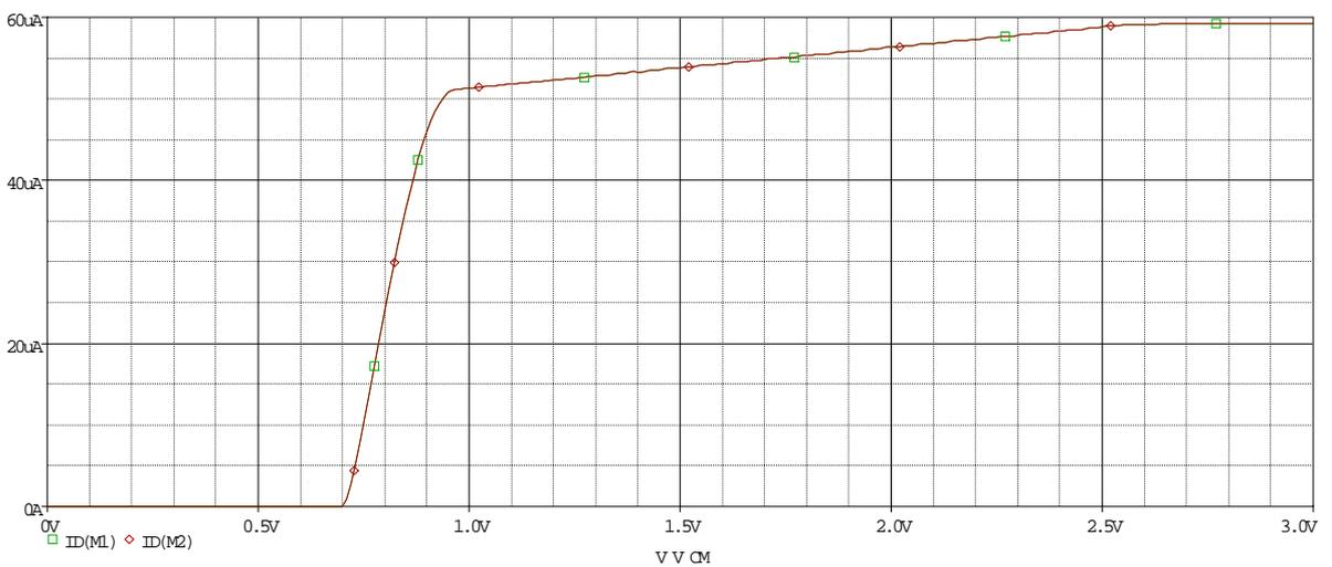
VCM sweep from 0V to 3V, voltage at connected source V(P), follows VCM when transistors in saturated region
