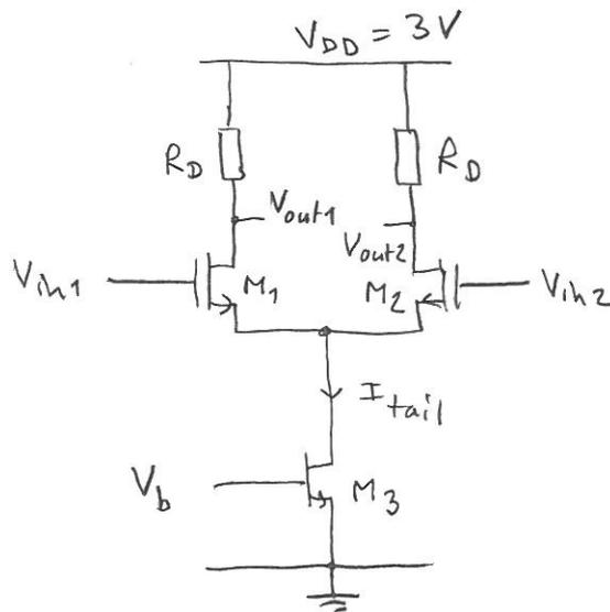
$$\frac{w}{L} = \frac{50\mu}{0,5\mu} \text{ for transistors } M_1 \text{ and } M_2$$
