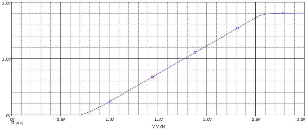
VCM sweep from 0V to 3V, voltage at output Vout1, Vout2
