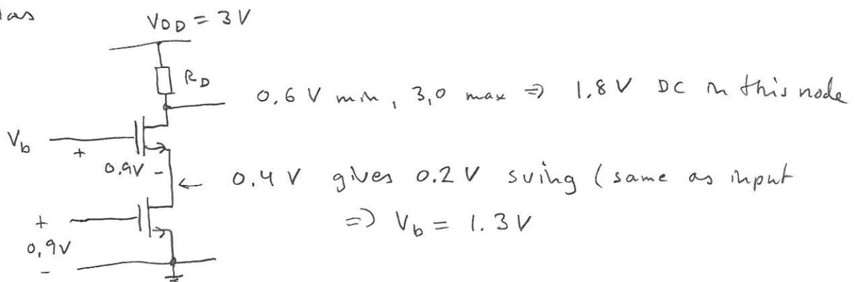
$$R_D = \frac{3 - 1,8}{394 \mu\text{A}} = 3,05 \text{ k}\Omega$$
