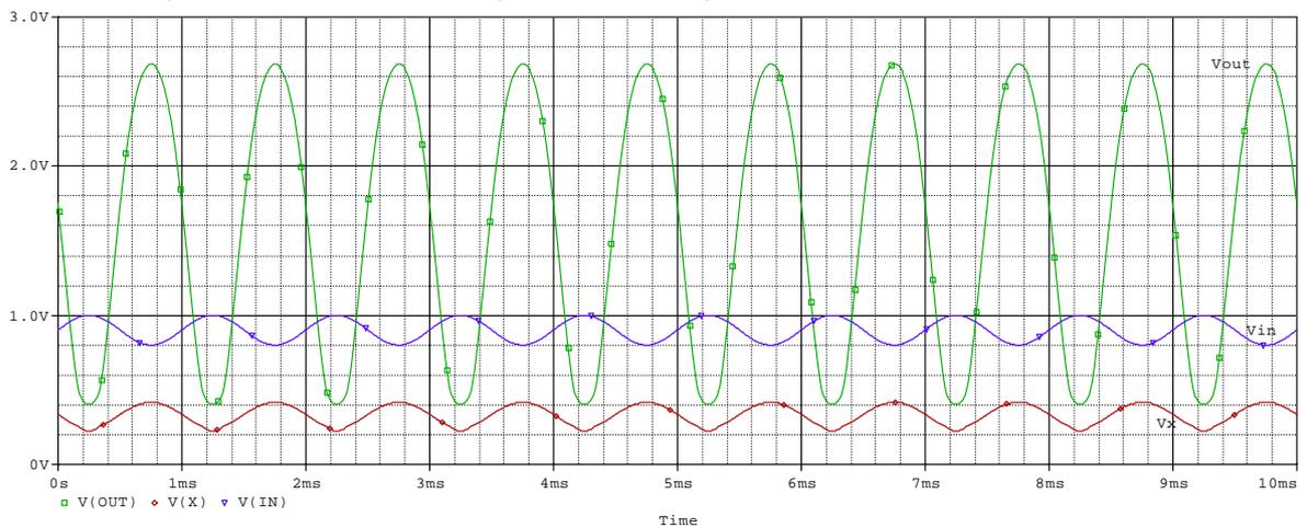
Output peak-to-peak 2.28 V, gain  $2.28/0.2 = 11.4$  large output signal. We can see that output is not a good sinus, distorted, non-linear amplifier.
