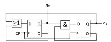
Sequence network starts in the state  $q_1q_0$  00. Analyze the circuit and give the sequence for the following four clockpulses.
