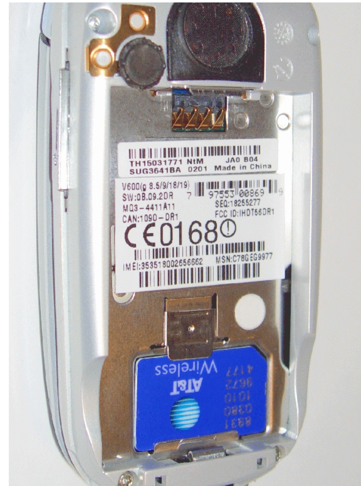
Figure 26: Phone without and with SIM card, note the IMEI number and other numbers printed inside the back of the phone.
