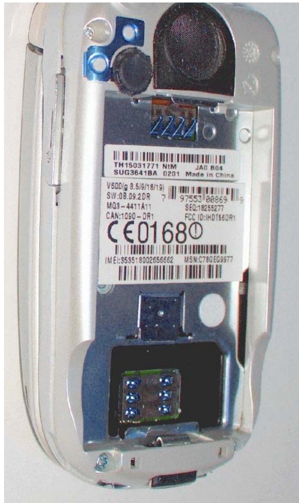
Figure 26: Phone without and with SIM card, note the IMEI number and other numbers printed inside the back of the phone.
