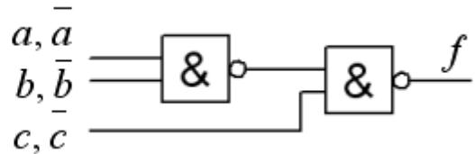
a) Write the logic function  $f = f(a, b, c)$  that is realized by the circuit.
