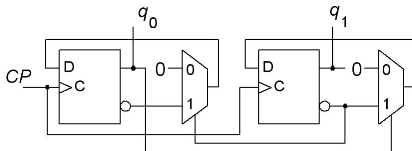
Sequential circuit shown above starts in the state  $q_1 q_0 = 00$ . Analyze the circuit and give the sequence of its states for the following four clock pulses.
