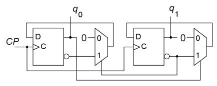
Sequential circuit shown above starts in the state  $q_1q_0\,$  00. Analyze the circuit and give the sequence of its states for the following four clock pulses.
