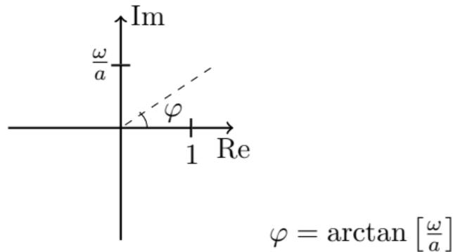
$$\Rightarrow \arg [G(i\omega)] = \arctan\left(\frac{\omega}{b}\right) - 90^\circ - \arctan\left(\frac{\omega}{a}\right)$$
