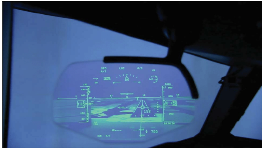
Figure 3.2: Illustration of HUD with EFVS in limited visual conditions [30]
